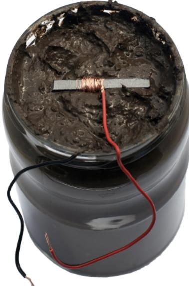
mud because it has to be in contact with the air. / Elektroda na vrhu kozarca mora samo delno potopljena v blato, saj mora ostati v stiku z zrakom.
