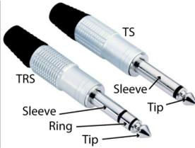
This image is of 6.5mm TRS & TS plugs. The tip, ring and sleeve are all separate connections. The sleeve connects to ground and the tip and ring to the mono or stereo channels.
